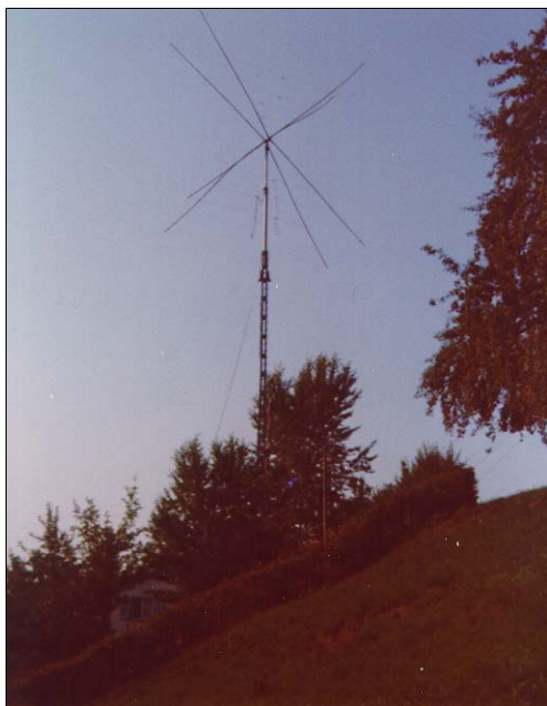
Dreiband 1 \frac{1}{2} Lambda-Quad: 20m, 15m, 10m
